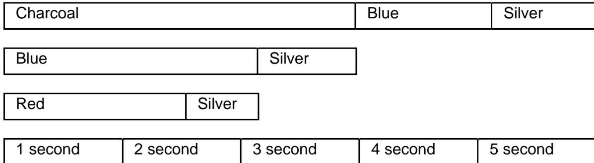
On paper this seems like a simple enough plan. You can easily imagine the flower blooming with successive layers of silver-tipped petals. The difficulty is in translating this time line into the design of stars of three different sizes that are layered with compositions of unequal burning speeds.
