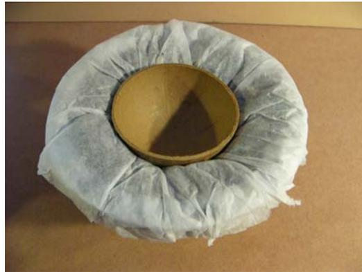
The other half of the Inner Petal is loaded with stars and burst. A cavity is formed with a 4" shell casing and the tissue paper keeps the burst in place. *Important:* The 4" casing is removed prior to joining together the Inner Petal hemispheres.
