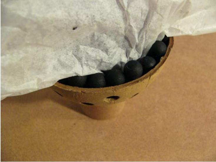
Stars are loaded in up to the edge of the hemisphere casing. Burst is added as needed to keep the stars pressed against the hemisphere wall.
