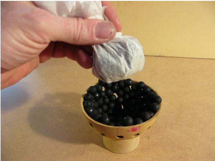
A small quantity of burst is placed in tissue paper and set atop stars. This technique keeps the tissue from ripping. Burst is added as required and then the tissue is folded back and pasted to the hemisphere exterior as was done with the other half.
