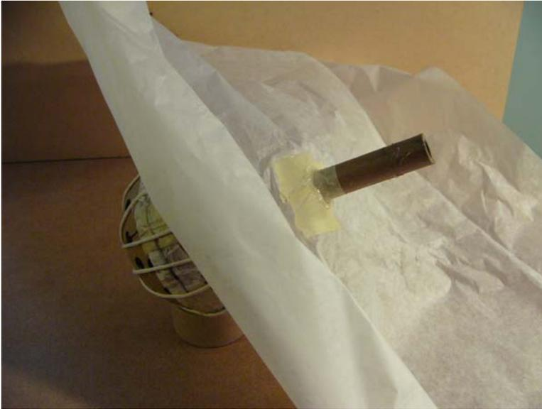
Large sheet of tissue paper (with masking tape gasket and hole) is affixed to pass-fire tube. The proper height for the tissue can be determined by pre-fitting the Inner Petal hemisphere so that it is level with the Pistil seam. The Tissue should be one star diameter higher.
