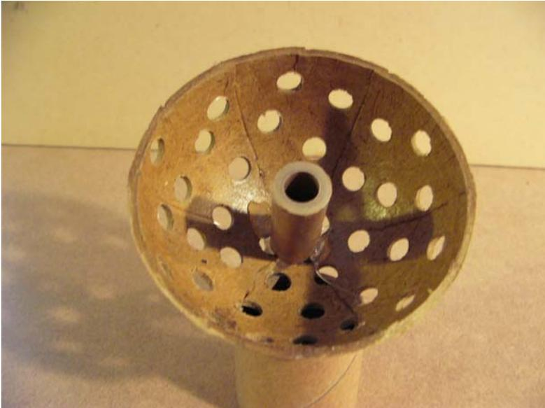
A 4" perforated pistil hemisphere with pass-fire tube glued in place. Pass fire-tube should be flush with pistil hemisphere top and its length equal to the interior depth of the final shell casing.
