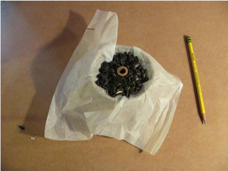
Burst is loaded to a level equal to the stars
