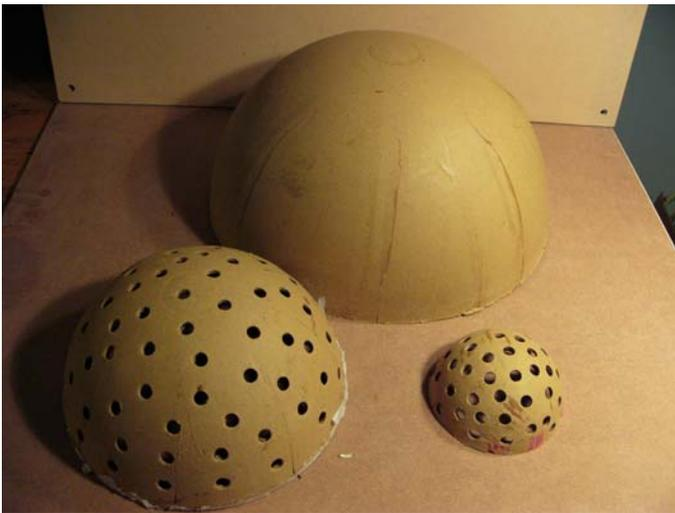
A 12" shell casing hemisphere (outer petal), an 8" inner petal perforated hemisphere, and a 4" perforated pistil hemisphere.
