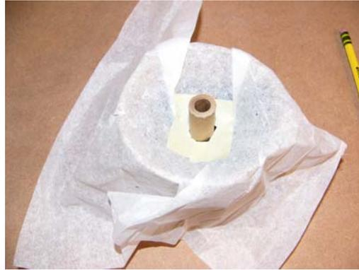
Tissue paper is prepared with masking tape gasket and hole for pass-fire tube and then inserted around pass-fire tube and over stars
