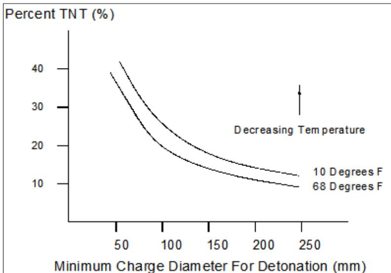
Effect of TNT Content on the Critical Diameter of TNT Slurries
