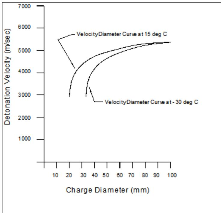
Effect of Temperature on a Small Diameter Watergel Explosive
