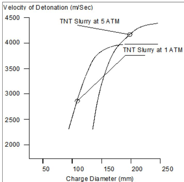
Effect of Hydrostatic Pressure on the Critical Diameter of a Watergel Explosive
