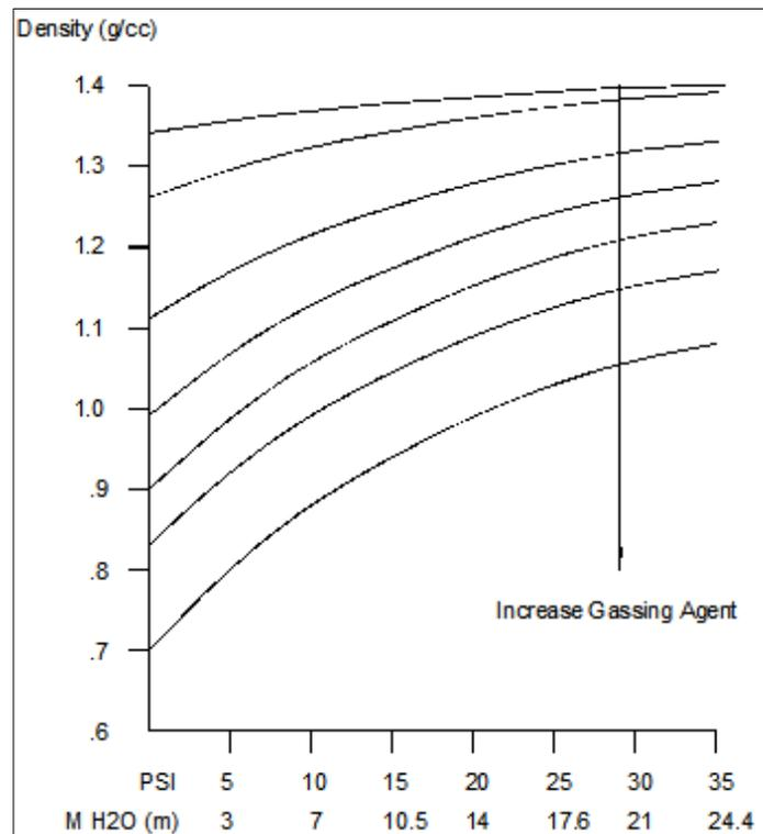
Effect of Hydrostatic Pressure and Gassing Agent Addition on the Density of an Aluminized Watergel
