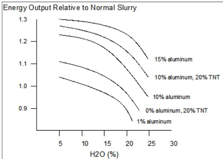
Effect of Water Content on Energy Output on Slurries
