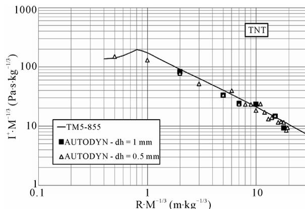
Figure 6. Positive impulse as a function of reduced distance for explosions of spherical TNT charges in free air.
