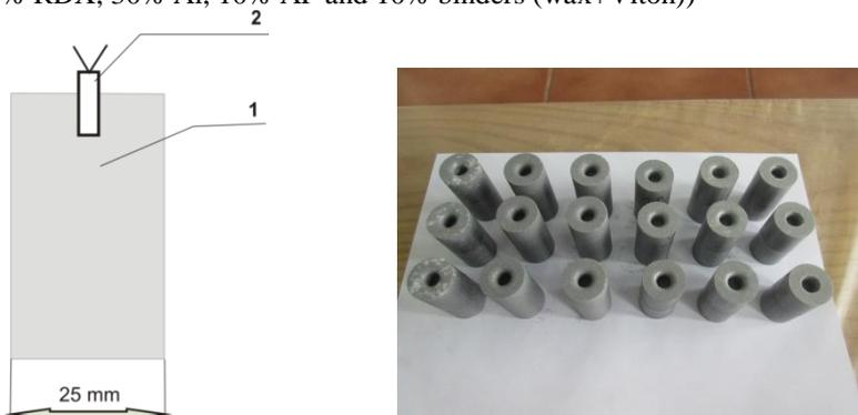
Fig. 2. Schematic and photo of the investigated pressed charges: 1 – composite, 2 – detonator
