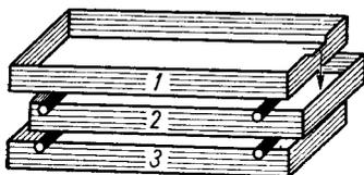
FIG. 79. Pans for crystallization of TNT (Pascal [5]).
