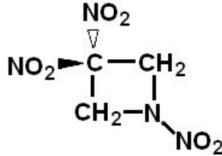
Trinitroazetidine (TNAZ) is unique in that it is based on a square ring. The strain from this configuration (which adds 37kcal/mol), as well as the high density from this geometric structure, lends increased power to the compound. It has a melting point of 101-103degC, and a density of 1.84 g/mL. The compound is considered melt-castable.
