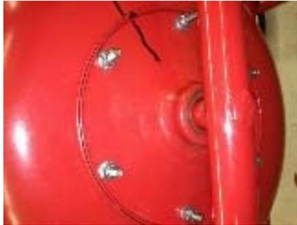
Step 8 The drum may be tilted a bit because the roller and the gear engagement is not exactly the same. Turn the barrel slowly by hand to be sure it turns freely. There may be 3 or fewer small bumps as the roller bumps over the button heads of the Screws. Plug in the roller and turn it on to check for free and quiet movement. Adjust as Necessary.
