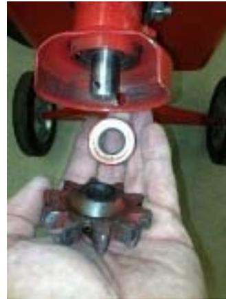
Step 5 Inspect the shaft for any damage done during the removal of the roll pin and gear.
