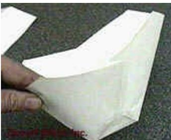
Larger shells require that you fashion a pouch out of paper. A single sheet triangular folded with the ends trimmed and taped makes an excellent pouch. Of course any design can be used just as long as it can be attached to the shell and it doesn't leak out the Lift Powder inside. The pouch is filled with the appropriate amount of Lift Powder and then securely taped to the bottom of the shell.
