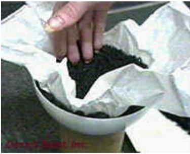
Hold the package of Hulls by the top and drop it into the shell, quickly spreading the Hulls up against the wall of stars. The Rice Hulls pressing on the stars will prevent them from falling in. The tissue paper merely prevents the stars from migrating into the center of the shell during transport or launch.
