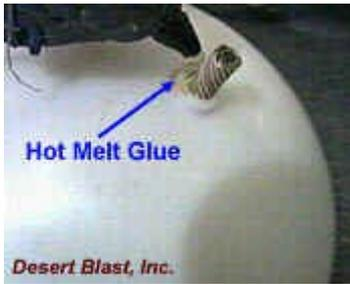
Using a Hot Melt Glue Gun, lay an even bead of glue around the base of the fuse sealing it to the casing. When cool, do the same on the inside of the shell. It is important that there be no gaps in the glue which could allow fire to enter the shell during launch.
