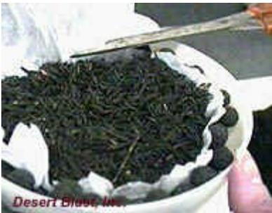
Trim the tissue paper so that it's under the lip of the shell casing. Add or remove some Rice Hulls until the shell is full to about 1/8" from the top. Check with a straight edge and be careful not to overfill, it would make it difficult to assemble the shell. Set this half of the shell aside when complete.
