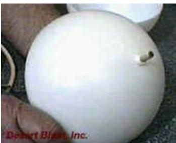
Insert a 1.25" long fuse into the bottom half of the shell, leaving about half the length sticking out the bottom of the shell.
