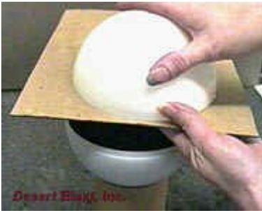
Place a thin piece of cardboard (like the kind you find on the back of note pads) on one half of the shell. Holding it in place, flip the shell over and lay it on the bottom half. Align the two halves, and slowly pull out the cardboard, snapping the two hemispheres together.
