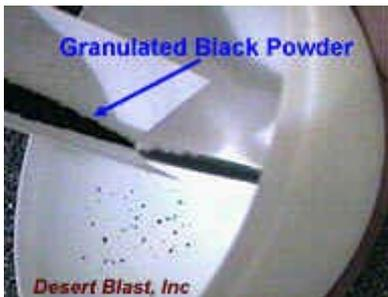
Fill the straw to within 1/4" of the top with granulated Black Powder. We use granulated Homemade Black Powder. Its manufacture is described in the [Black Powder & Rice Hulls](#) section. Commercial 3FG or similar may also be used.
