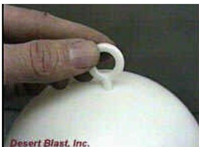
Flip the shell over, dip the fuse ring (that came with your shell casing) in some solvent and insert it in the top hole. The fuse ring will support the shell as it is loaded into the Mortar.
