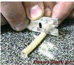
It is important that time fuse is cut with a blade and not a scissor-type device. The powder core is somewhat fragile and if cut with a scissors or similar device the end is crushed (to varying degrees) and the powder loosened from its packed state, increasing its burn rate.
