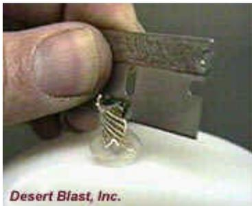
Using a razor blade, slice the Time Fuse in half to a depth of about 1/4"
