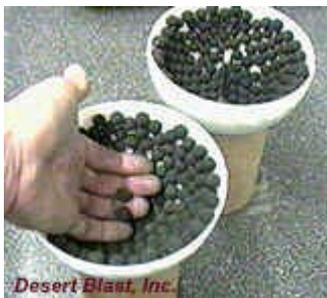
Continue loading until both halves of the shell have a layer of stars along the inside. Do not load the stars all the way up to the rim. There is a small lip on shell halves that must fit together, so leave a space of about 1/4" from the rim on both halves.
