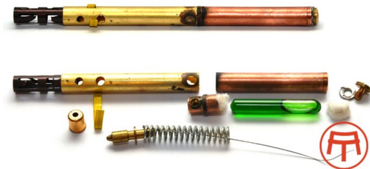
*wire running along the ampoule of copper chloride. The cotton wads serves a dual purpose; to protect the ampoule against hard handling during transport and when the ampoule is crushed absorb the copper chloride to ensure that the wire is fully submerged regardless of the position of the pencil. Also notice the circular inspection hole next to the safety strip. Shown from left: primer, firing pin, coil spring, ampoule, lead disk, retaining screw and in between the steel wire.*
