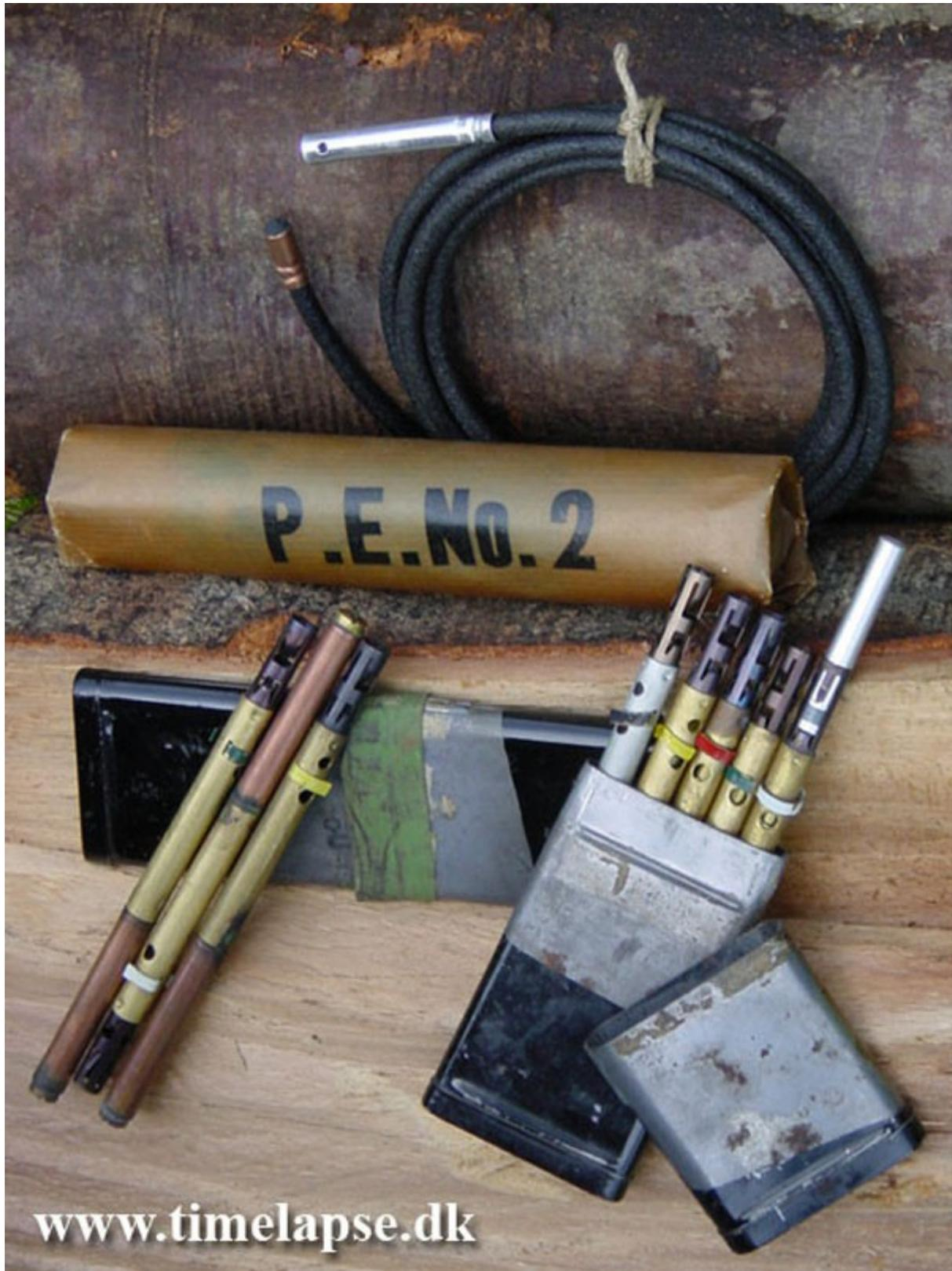
*The photo shows two stamped tin boxes each containing 5 Time-pencils that was airdropped to the Danish resistance during the Second World War. On top a roll of Bickford fuse with a crimped detonator and a safety match igniter all ready to go. Note the inserted No. 27 detonator in the white time-pencil to the right. For illustration purposes I have mixed the various colors.*
