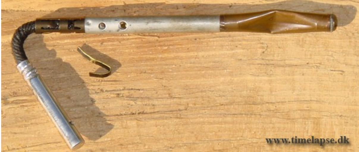
at the end, timed for action within 10 minutes. The advantage in using the Bickford fuse is that the operator will have a safety margin if the switch should fail and fire in the second the safety strip is removed. A Bickford fuse burns 0.40 inch (1 centimetre) per second leaving enough time to extract the detonator from the explosive. Note the extracted black safety strip and the two inspections holes.
