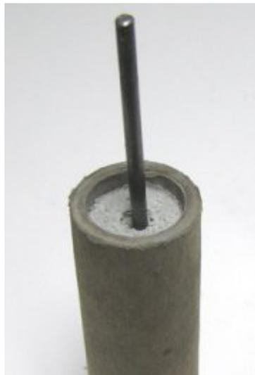
Here is how the pass-through hole is made. A wire is placed on top of the delay, clay is poured around it, the whole thing is tamped with a hollow drift (same one that is used to tamp the fuel). Notice the clay pulled away around the wire. That is because it wasn't pressed in hard enough. Below is another picture of a couple of 5/8" motors that had the bulkhead pressed on. Nice and clean, eh?
