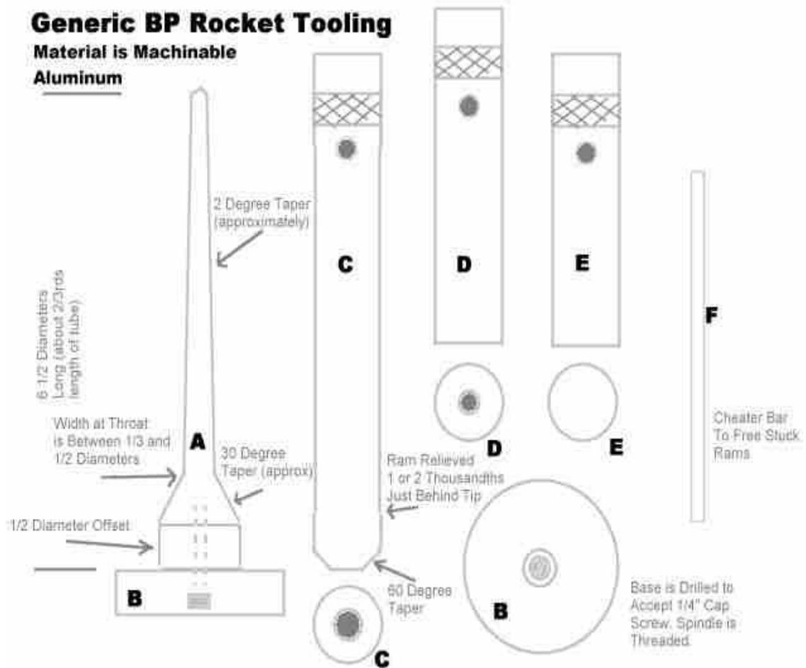
Above is a general guide for creating BP rocket tooling from aluminum stock. You can vary these measurements slightly depending on your particular need. If you are just starting to make your tooling, try to get it close to these measurements and vary your fuel to get the performance you desire. This tooling works fine for nozzleless designs, too.
