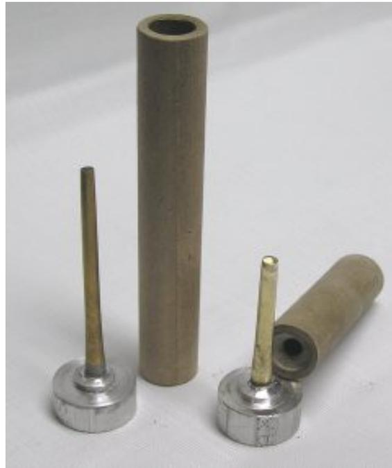
Above are some machined rocket tools made from scrap material in a shop. You can also just make the tooling from wooden doweling. The longer core on the left will require a much cooler fuel ([RP](#) or similar). The one on the right can take a hotter fuel. Neither set of tools has a proper convergent/divergent angle but they still fly swell!
