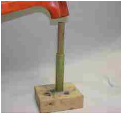
For smaller rockets (1/4" to 1/2") I use a dead blow hammer or arbor press depending on the composition - ramming should only be done with BP! If your BP is granular (pulverone or similar) then you need to compact it harder to consolidate the granules into one long grain (see the fuel section below). Generally, powdered BP (meal powder) compacts easiest - especially if you use small increments.
