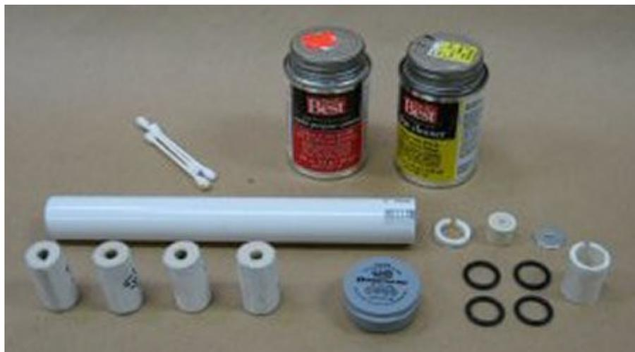
**Preparing for final assembly of F motor**
