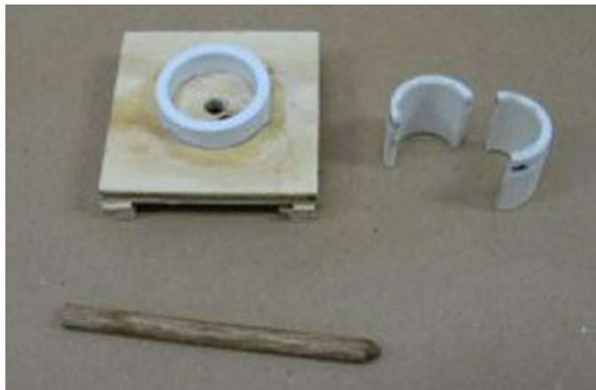
**Casting tube, support guides and coring tool**
