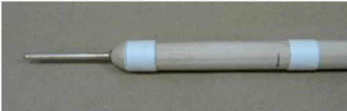
**Masking tape on nozzle mold**
