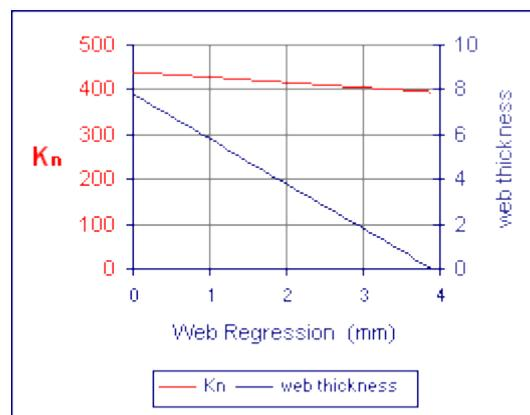
Figure 4 -  $K_n$  as a function of web thickness
