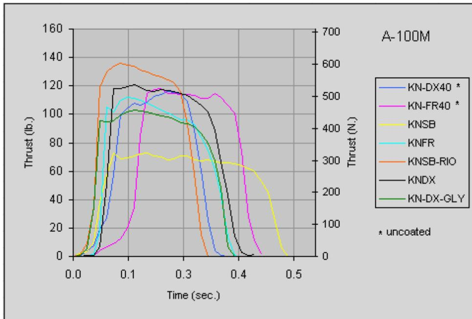
Figure 5 - Thrust versus time plots
