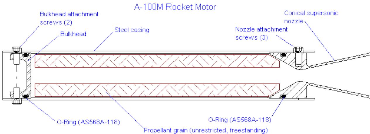
**Figure 3** - Cross-sectional view of the *A-100M* motor assembly
