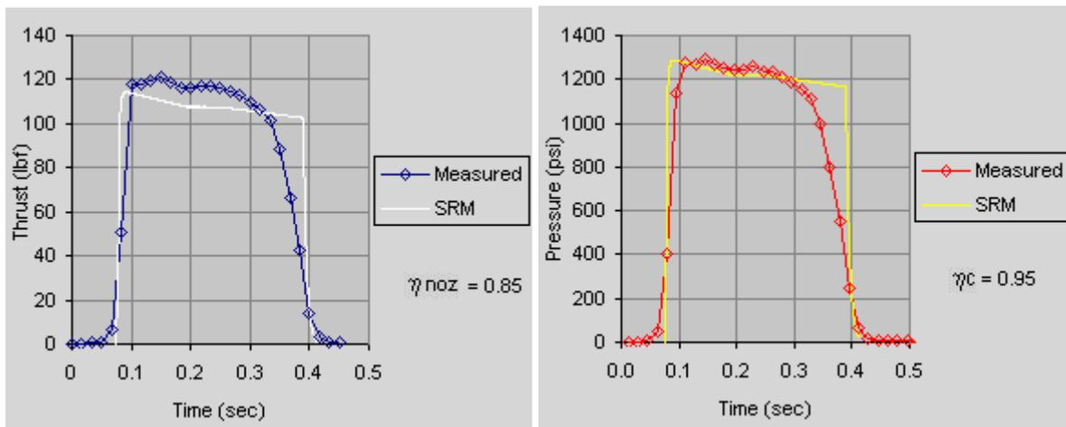
**Figure 7 - Measured versus SRM prediction**
