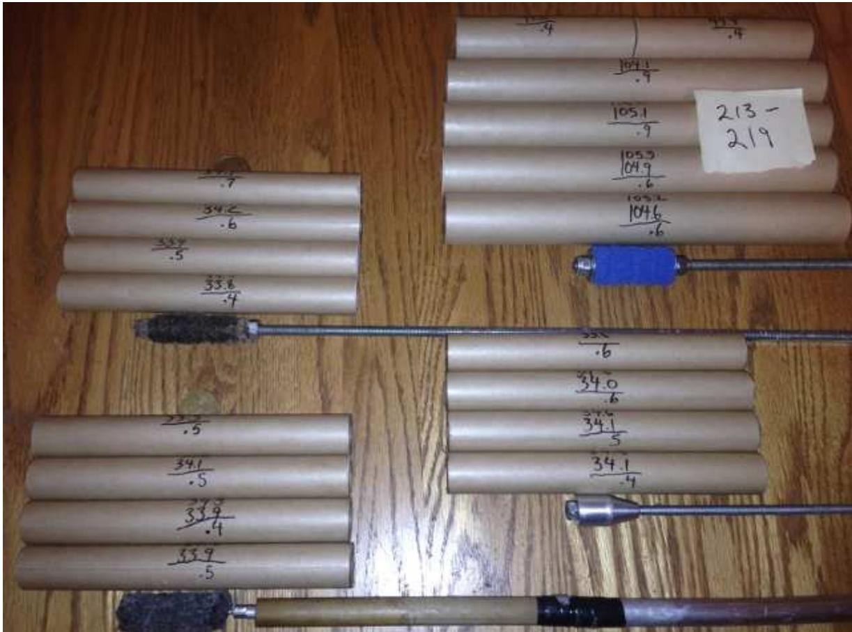
The numbers on the tubes indicate the weights of the tube before and after waxing, and the difference in grams. There is not much difference in the amount of wax applied with the different daubers. For a 1-pound tube 7 1/2" long, about half a gram of paraffin is applied. The dauber on the upper left is my original one, made by wrapping jute around a threaded rod and putting nuts on the ends.
