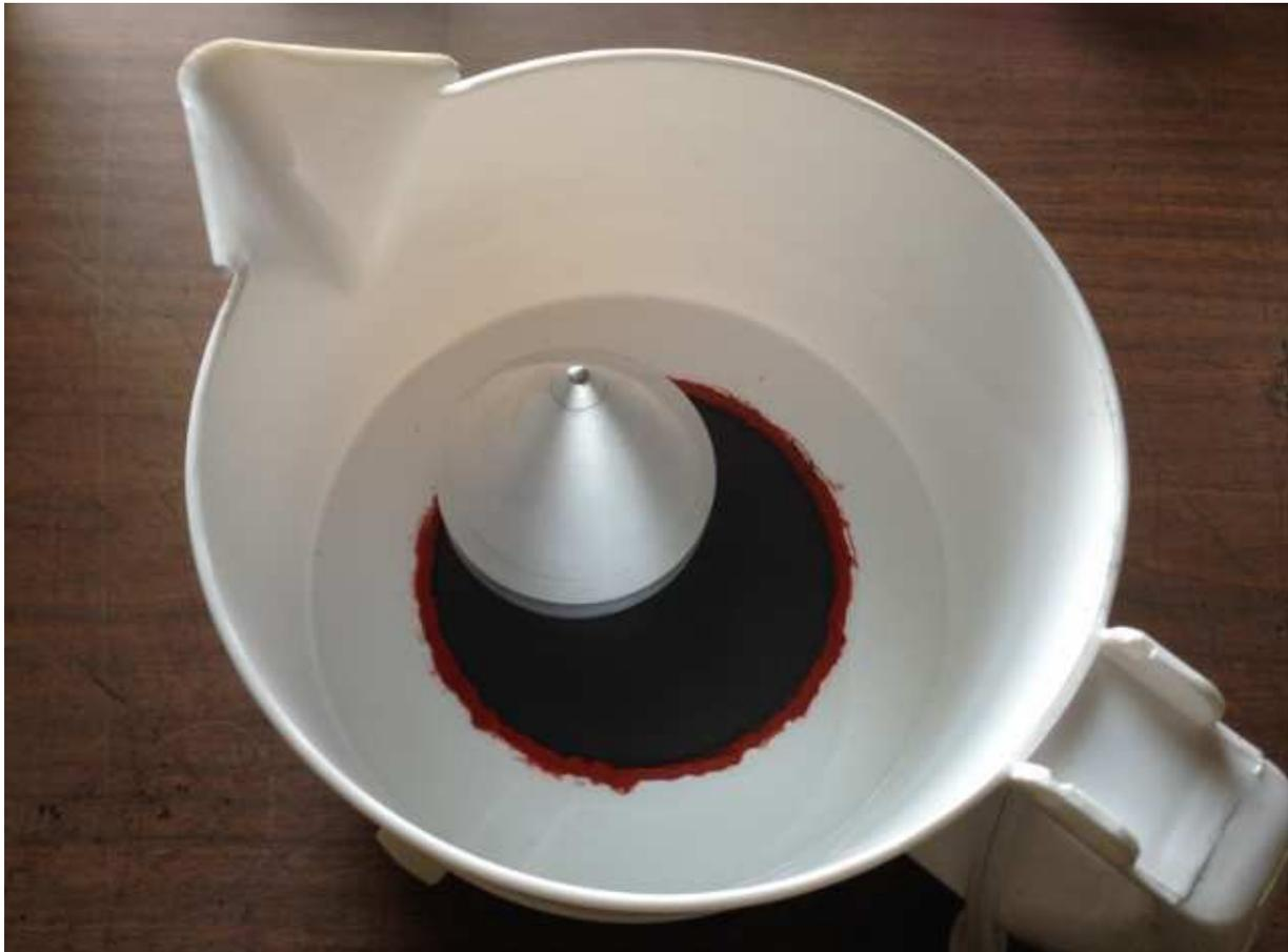
Please note, however, that these cheap pots don't stand up to the melted wax for very long. Better-quality pots are needed. I used red high-temperature silicone to try to delay the inevitable, since I had already purchased these before I found out that they would leak. Ned has since stepped up to Presto Brand pots made of aluminum.
