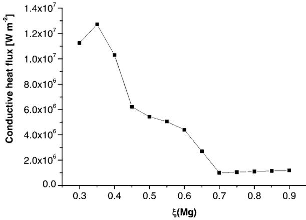
**Figure 10.** Heat flux via heat transfer from the gas phase to the burning surface.
