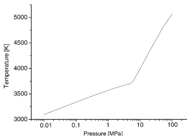
**Figure 2.** Variation of the adiabatic flame temperature at  $\xi(\text{Mg}) = 0.32$  versus pressure with  $p = 0.01 - 10$  MPa.
