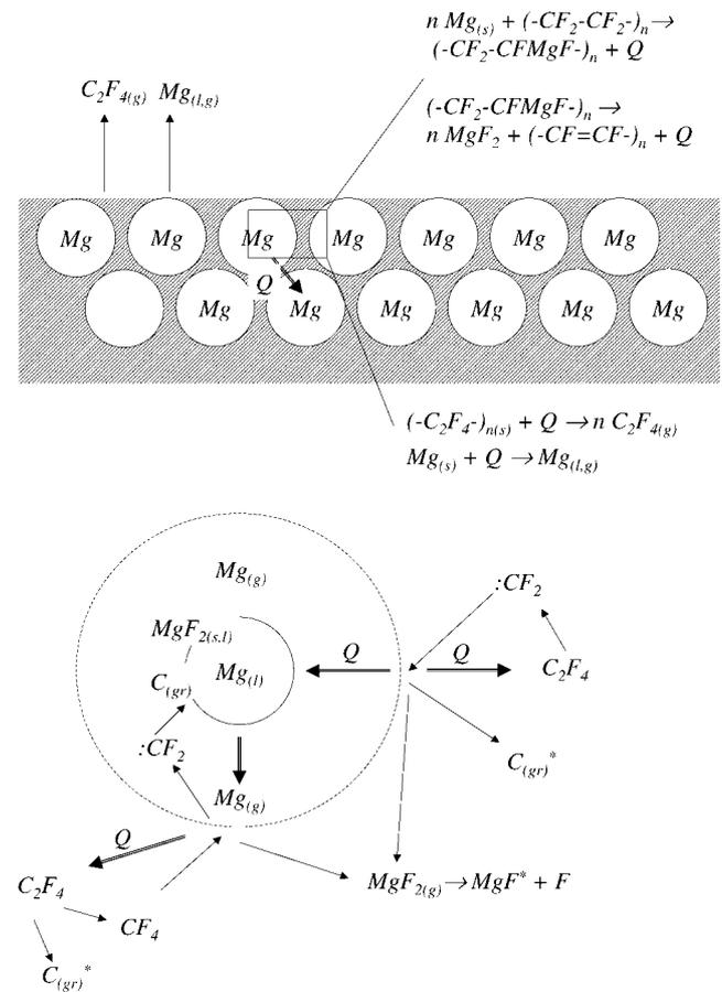
Scheme 2. Proposed reaction path of MT combustion in both condensed phase a) and gas phase b).
