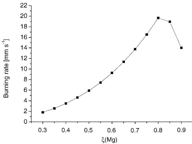
**Figure 9.** Propagation rate of the preignition reaction in the condensed phase.
