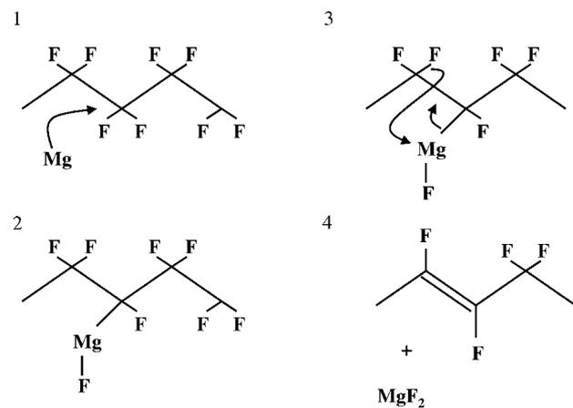
Scheme 1. Proposed reductive elimination of fluorine from PTFE applying magnesium under DSC experiment conditions.
