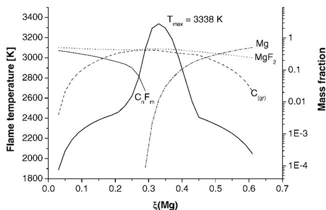
Figure 1. Flame temperatures and weight fractions of major combustion products at 0.1 MPa.
