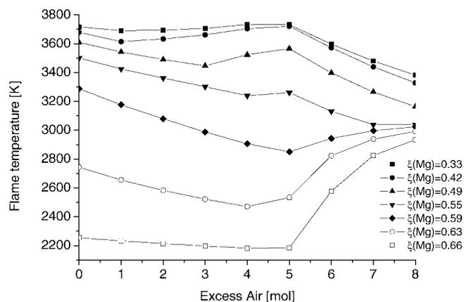
**Figure 3.** Variation of the adiabatic flame temperature at various  $\xi(\text{Mg})$  as function of excess air added on a per mole magnesium basis.
