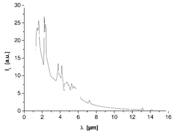
Figure 5. FTIR-emission spectrum of MTV at  $\xi(\text{Mg})=0.32$ .
