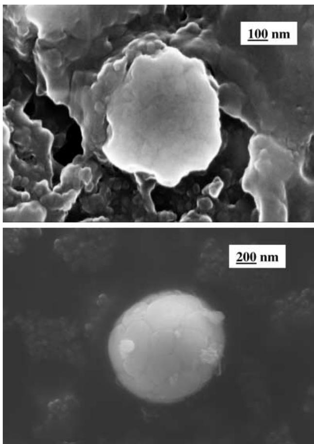
Figure 6. a and 6b.  $\text{MgF}_2$  combustion particles.
