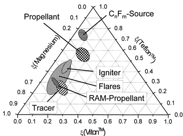
**Figure 1.** Ternary MTV diagram showing various applications.
