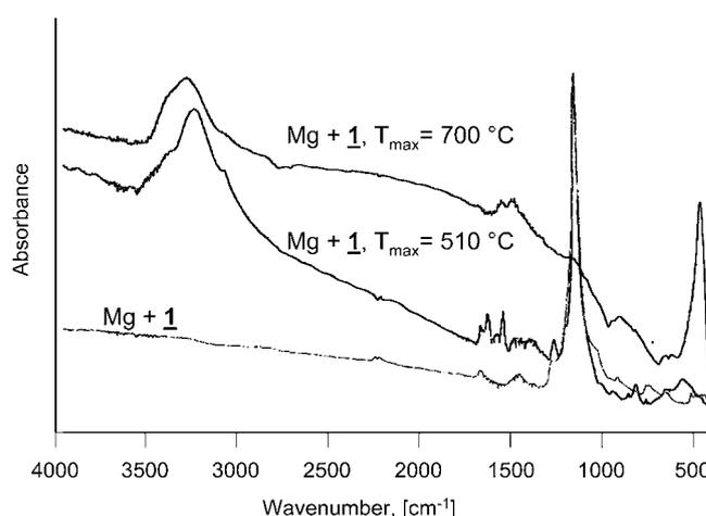
**Figure 3.** FTIR spectra of pyrolant and DSC residues
