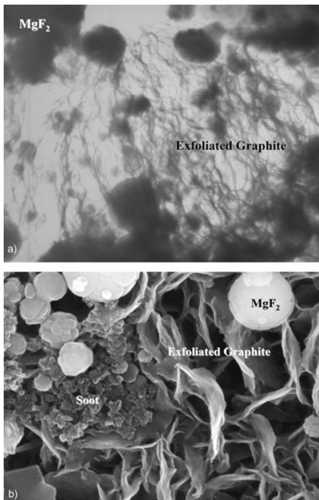
Figure 4. TEM a) and HREM b) picture of combustion product
