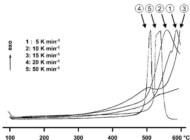
**Figure 2.** DSC plots of pyrolant at 5, 10, 15, 20 and 50 K min<sup>-1</sup>.
