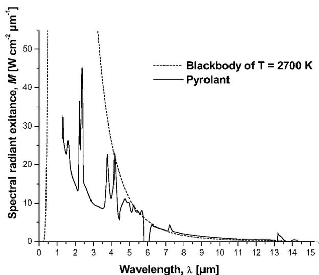
**Figure 7.** Spectral radiant exitance of pyrolant and blackbody having  $T = 2700 \text{ K}$
