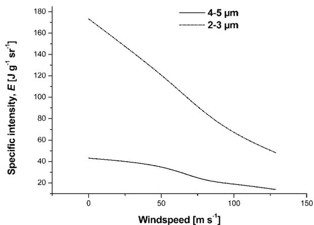
**Figure 8.** Specific intensity  $E_{\lambda}$  of pyrolant under static and dynamic conditions at two bands
