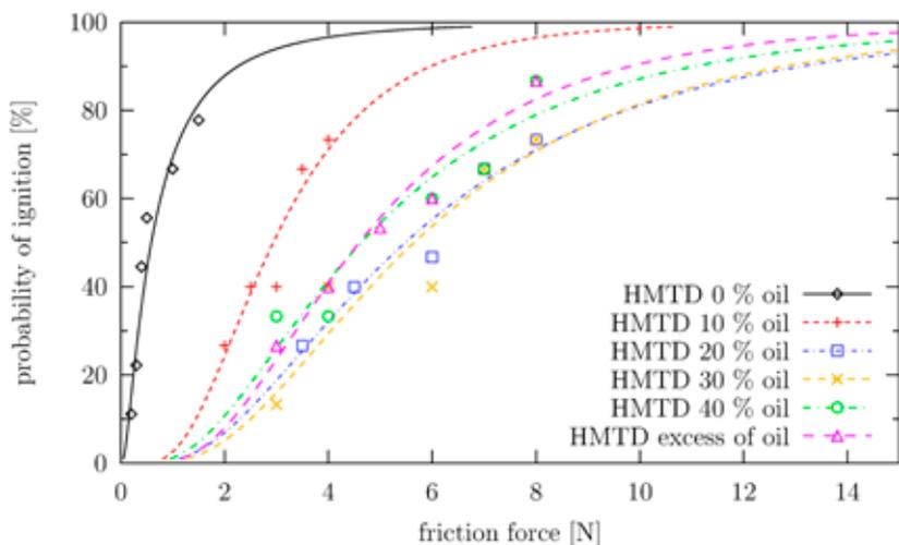
**Figure 6.** Sensitivity to friction of HMTD with oil WD-40.
