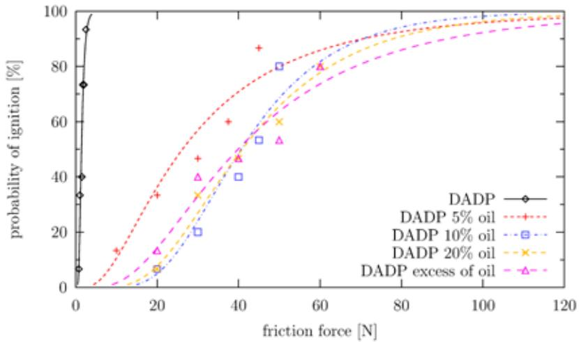
**Figure 4.** Sensitivity to friction of DADP with oil WD-40.
