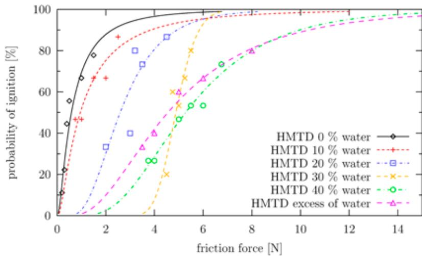
**Figure 5.** Sensitivity to friction of HMTD with water.
