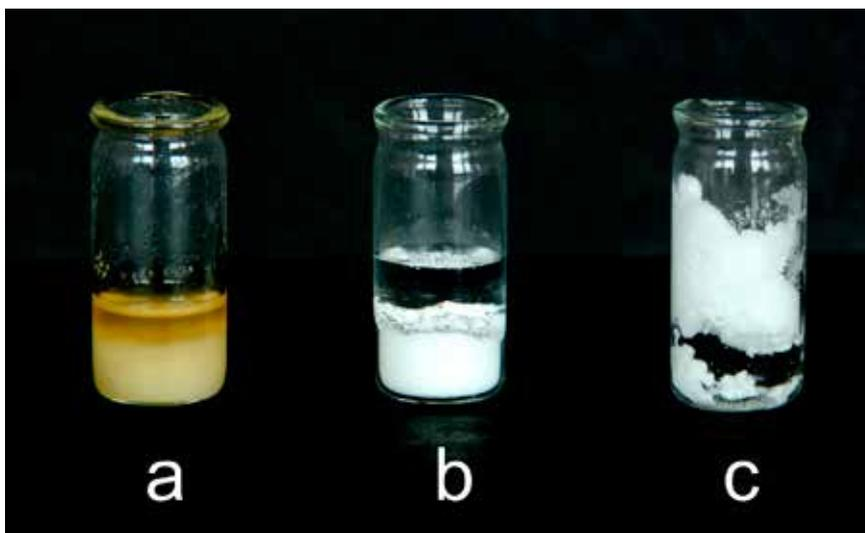
**Figure 10.** The addition of an excess of liquid to TATP: (a) TATP with oil WD-40 (just sprayed, without mixing), (b) TATP with water just after the addition, water does not penetrate the layer of TATP, (c) TATP with water during mixing, the TATP and water phases are still separated.
