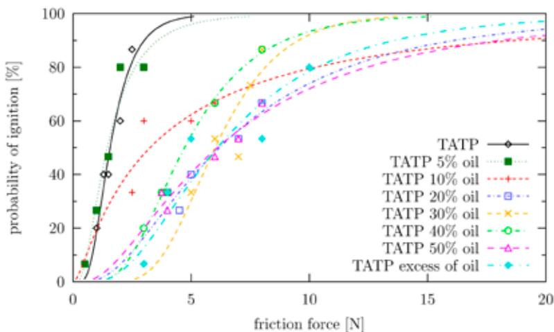
**Figure 2.** Sensitivity to friction of TATP with oil WD-40.
