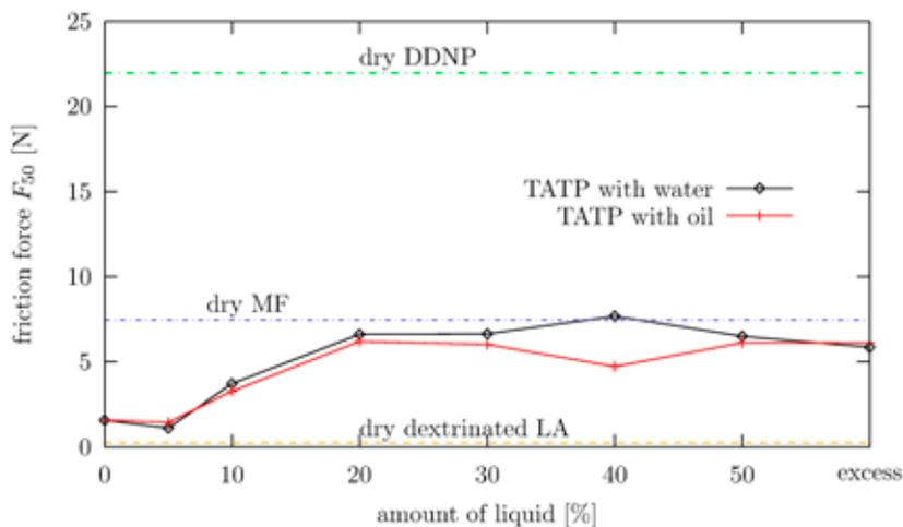
**Figure 7.** Decrease in the sensitivity to friction ( $F_{50}$ ) of TATP (LA – lead azide, MF – mercury fulminate, DDNP – 2-diazo-4,6-dinitrophenol).
