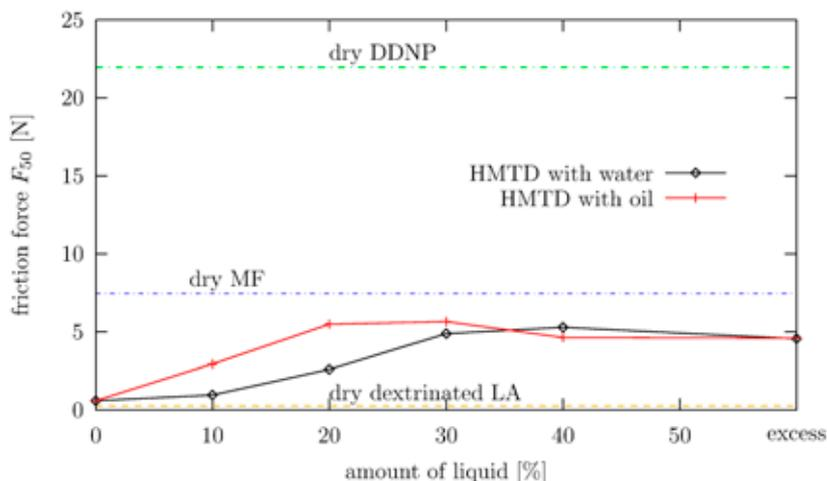
**Figure 9.** Decrease in the sensitivity to friction ( $F_{50}$ ) of HMTD (LA – lead azide, MF – mercury fulminate, DDNP – 2-diazo-4,6-dinitrophenol).
