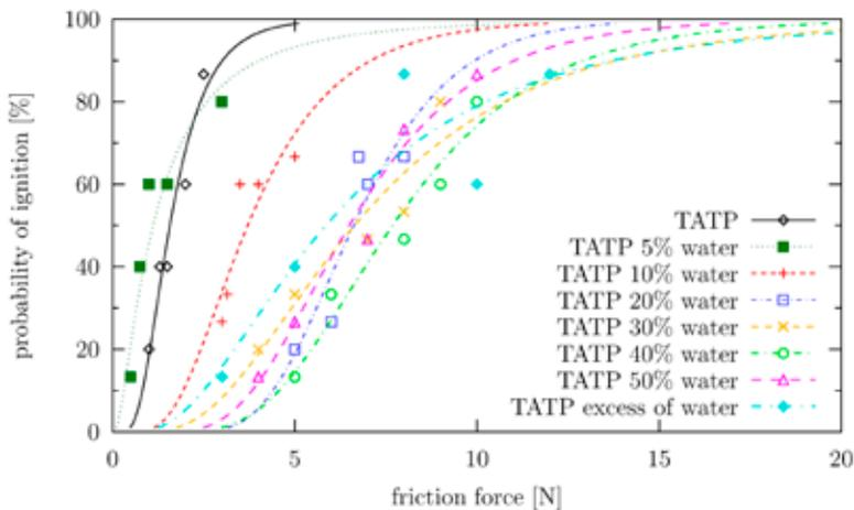
**Figure 1.** Sensitivity to friction of TATP with water.
