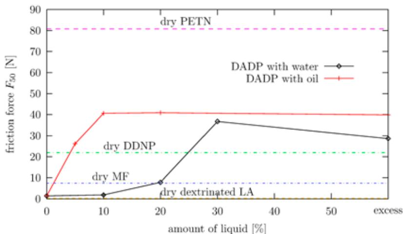
**Figure 8.** Decrease in the sensitivity to friction ( $F_{50}$ ) of DADP (LA – lead azide, MF – mercury fulminate, DDNP – 2-diazo-4,6-dinitrophenol, PETN – pentaerythritol tetranitrate).
