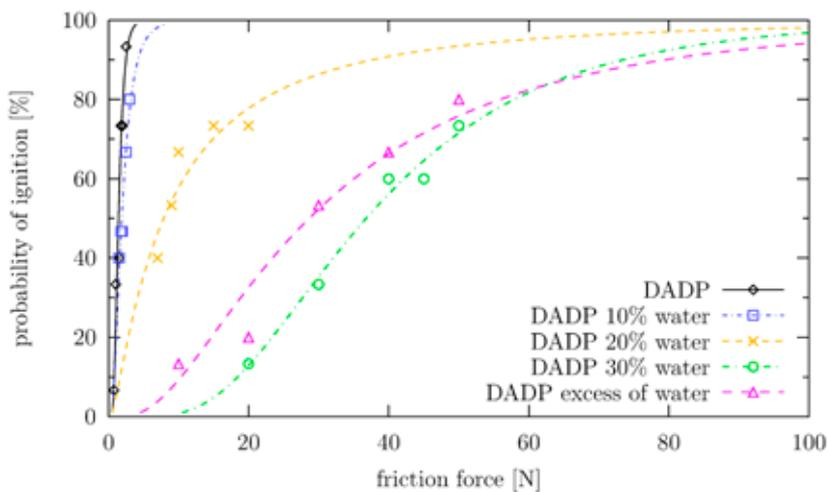
**Figure 3.** Sensitivity to friction of DADP with water.
