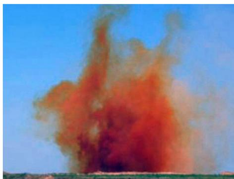
**Fig. 1.** Cloud of nitrogen oxides formed during rock blasting [8]
