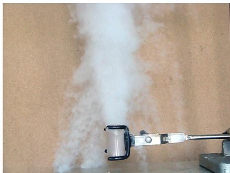
**Fig. 3.** Decomposition of a sample of HTP caused by potassium permanganate
