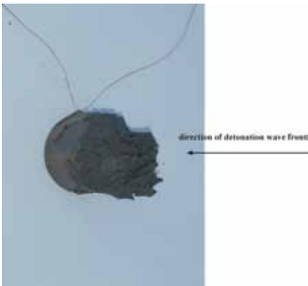
Figure 4. Detonation failure in PBX-4
