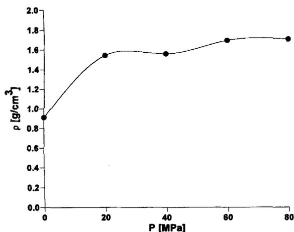
**Figure 1.** P-ρ Diagram of NHN**Table 5.** Sensitivity Data of NHN
