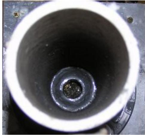
Epoxy coated chamber inside mortar
