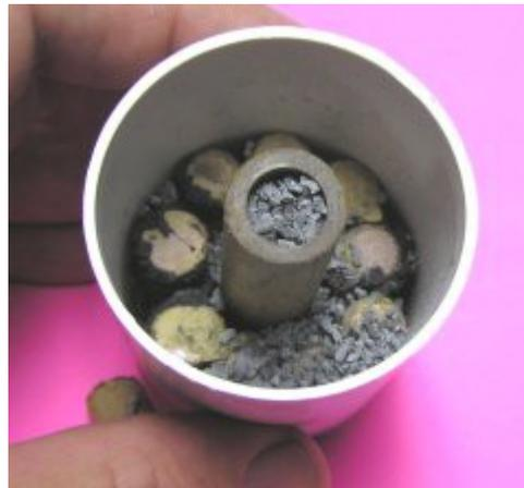
Middle tube will be removed - it's there to hold lower layer of hummers in while they're being inserted. Note primed sides
