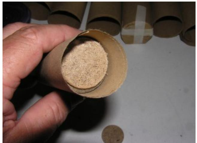
Insert the fiberboard plug into the tube
