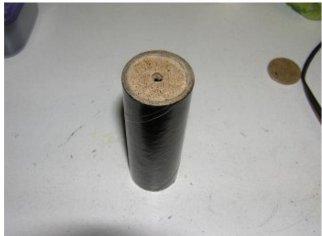
Here is a homemade case former - it is just a 1 1/2" tube with a fiberboard plug with a hole in it (to stop from
