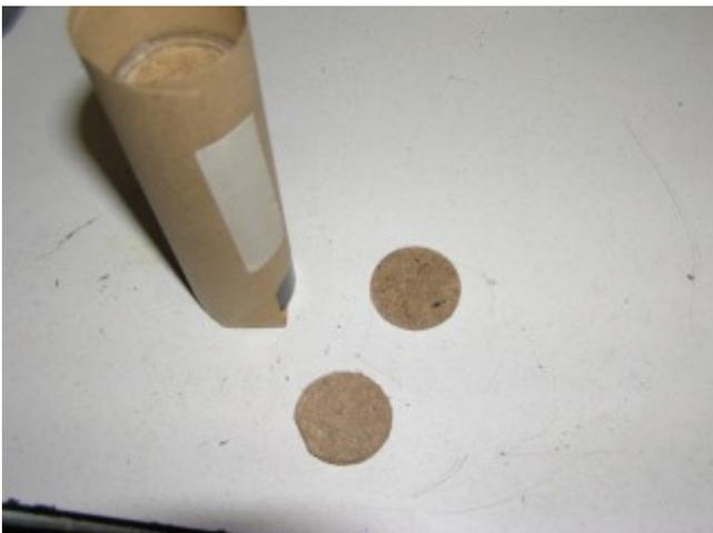
Use a fiber plug for the base. These were cut out with a hole saw - they don't have to be precise (and these aren't)
