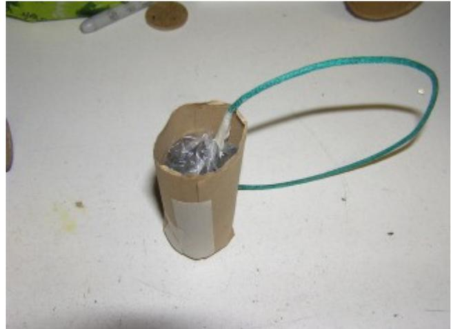
Put the star bag into the case. Note how the tape binds the baggy and fuse together - this stops the fuse from pulling out.
