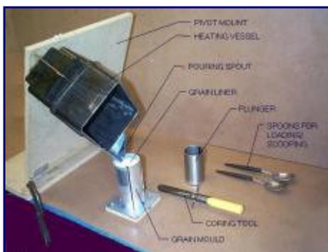
Figure 5 -- Casting setup for KNDX, employing 'tilt-table' for the heating vessel.
