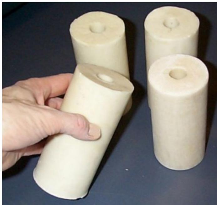
Figure 6 -- Cast *Lambda* KNDX propellant grain segments
