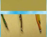
This is what it looks like when both are soldered. This igniter is now ready for dipping into the pyrogen and then it will be done.
