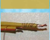
Next, push the two lead wires together and then the end of the ignition wire around the insulated part of the longer lead and wrap onto the bare part of that wire.
