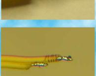
Here is another variation if you are experienced at soldering and have wire wrap. The insulation doesn't melt quickly. For a little added strength against breaking the bridge wire between the two leads, wrap two or three wraps around the shorter lead where it is stripped and the longer lead's insulation as shown.
