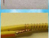
If you are experienced at soldering and your insulation doesn't melt at soldering temperatures, you can wrap both wires before soldering. My twisted pair wire melts so I have to solder the short lead first. I can solder both at the same time on the shooters wire. Here again, the long tail on the igniter wire that is necessary for hanging onto when wrapping the first lead wire should be clipped off.
