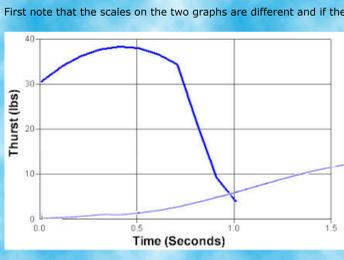
The simulation doesn't even start until it starts building thrust. Before that, it is just burning off propellant with nothing happening. The total area under the curves is the total impulse so you can see that there is significantly less when it takes time to build up to pressure. By the time it does start building up pressure, there isn't enough propellant left to build up to operating pressure.
