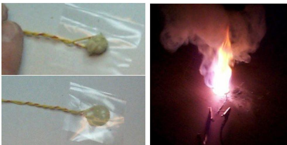
Figure 7 -- *Top left: Applying pyrolant*
