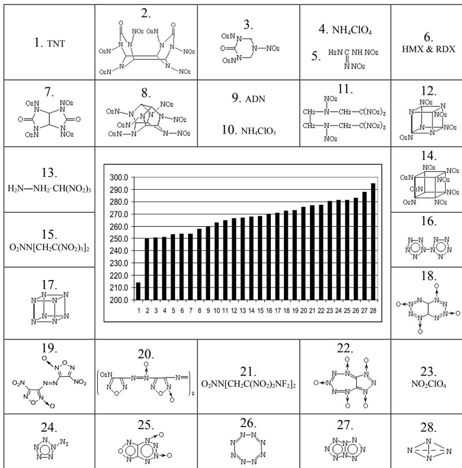
**Figure 1.**  $I_{sp}$  values (at pressure in the combustion chamber and in the exit nozzle section being 40 and 1 atm, respectively) for optimal mixture of the oxidizer with hydrazine.
