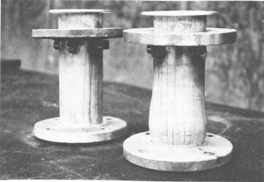
**Fig. 5.** Damage to reactor vessel (right) caused by spontaneous detonation of mixture of Bachmann chemicals.
