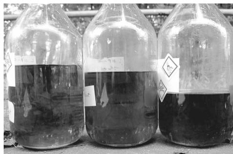
**Figure 2.** Prepared LMP-103S samples contaminated with metal ions.
