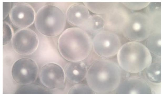
Figure 13. Improved 100% dense ADN prills with reduced sensitivity.
