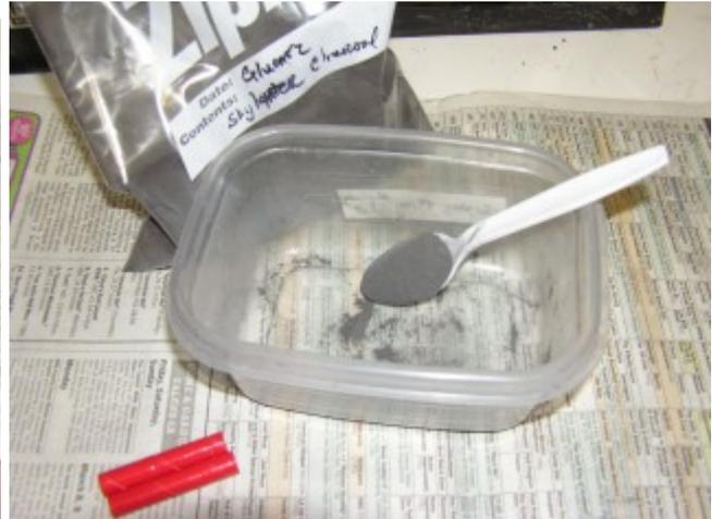
We'll do an example using a 1/4" cracker case and a teaspoon of mix (which would make several fuses)
