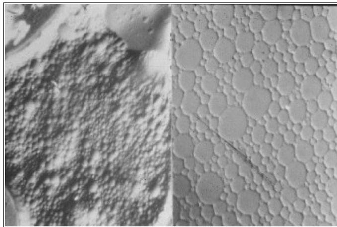
Emulsion Explosive Showing Normal Cell Size No Magnification on Left, 100X Magnification on Right
