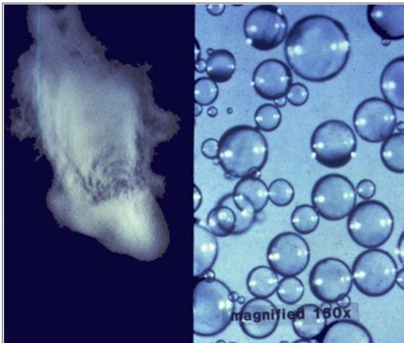
Microballoons (Hollow Glass Spheres) - 1<sup>st</sup> at normal magnification, 2<sup>nd</sup> at 160X
