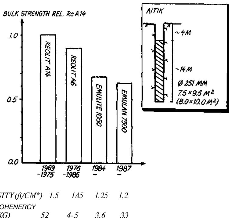
Figure 4. Bulk strength relative Reolit A14.
