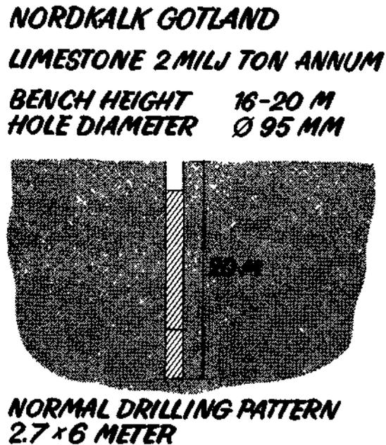
Figure 5. Blasting geometry at Nordkalk.
