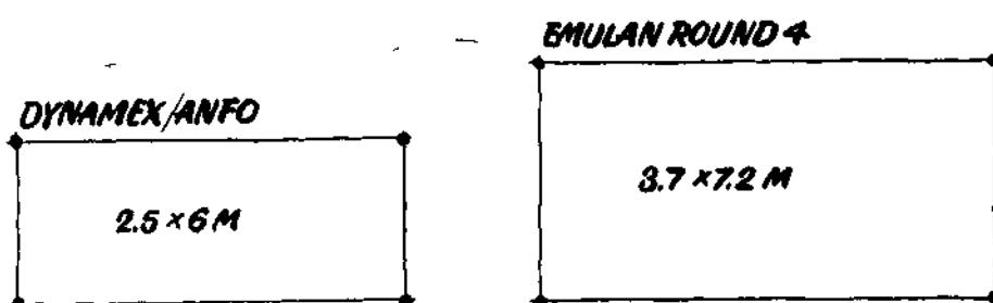
Figure 6. Original and final drillpattern after change of explosive.
