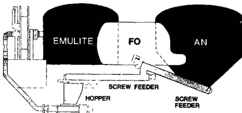
Figure 8. Schematic layout of EMULITE/EMULAN bulk truck.
