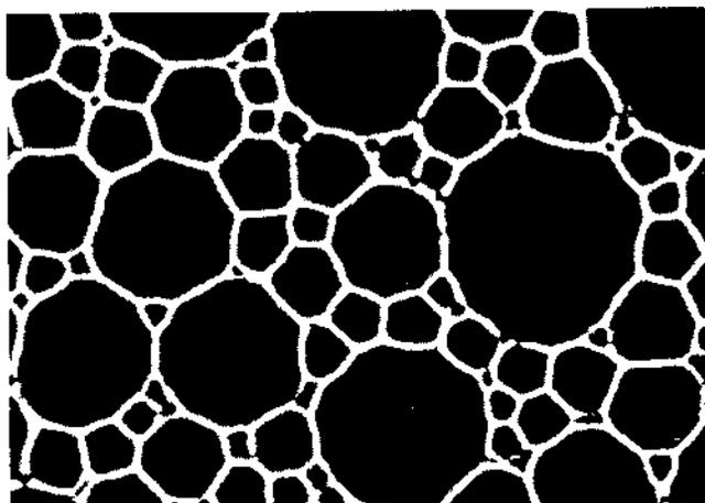
Figure 1. Structure of an emulsion seen through a microscope.
