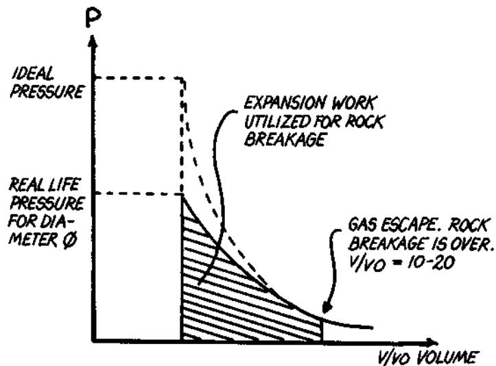
Figure 9. Schematic description of ideal and non-ideal behaviour.
