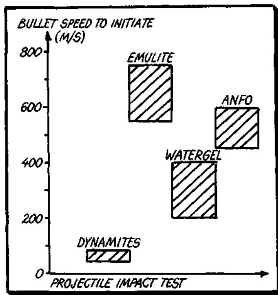
Figure 2. Sensitivity for some commercial explosives in the projectile impact test.
