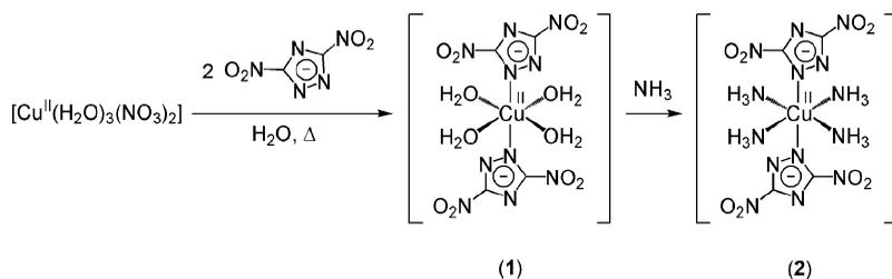
**Figure 2.** Synthesis scheme for tetraamminebis(3,5-dinitro-1,2,4-triazolato- $N^1$ )copper(II) (**2**).
