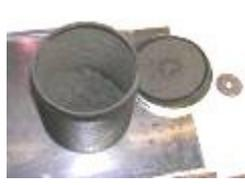
Drop in ball mill and mill 24 hours (if using a rock tumbler)
