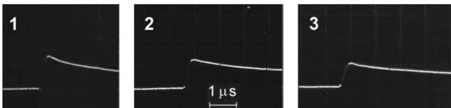
**Figure 3.** Mass velocity records of ammonals (sample 1, 2 and 3 – respectively to Table 1).
