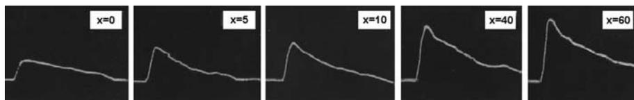
**Figure 7.** Mass velocity records illustrating the development of the detonation wave in the charge of hydro-ammonal with 8% of flaked aluminium ( $x$  – distance in the charge in mm).
