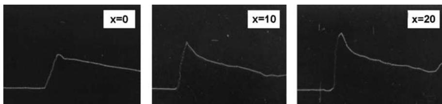
**Figure 5.** Mass velocity records illustrating the development of the detonation wave in the charge of ammonal ( $x$  – distance in the charge in mm).
