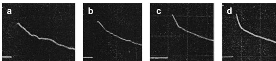
**Figure 6.** Mass velocity records of hydro-ammonals containing 4, 6, 8 and 10% of flaked aluminium (a – d) respectively.
