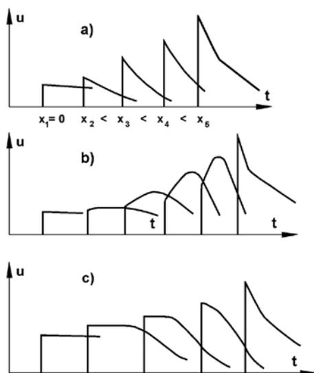
**Figure 2.** Profiles of a mass velocity during development of detonation in heterogeneous explosives [11]; TNT of density  $0.9 \text{ g/cm}^3$  (a), pressed TNT of density  $1.6 \text{ g/cm}^3$  (b), casted TNT of density  $1.6 \text{ g/cm}^3$  (c).
