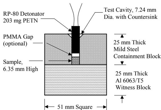
**Figure 1.** SSRT test arrangement.
