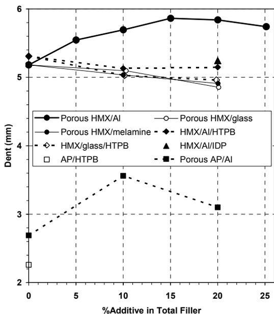
FIGURE 2. Effects of adding Al versus inerts and fuels to 60 %vol HMX or to 60 %vol AP.
