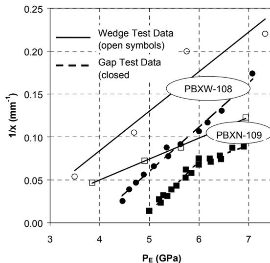
Figure 3. Run distance to detonation in gap and wedge tests for PBXW-108 and PBXN-109 from Figure 3 of Reference 9.
