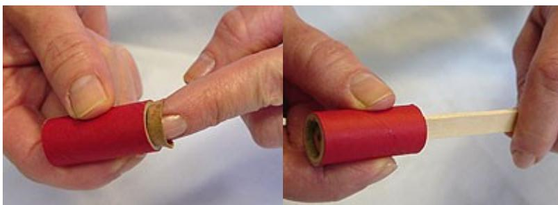
This end plug is going to be the bottom of the shell (projectile), and to make it strong enough to withstand the blast of launching it out of the mortar, we're going to use it backwards in the tube and reinforce it. Be sure to punch a hole in it for the fuse. Press the end plug in one end of the tube, and using a small stick or pencil, push the plug all the way to the other end, leaving a full 1/2" of space above it. This space is important, it will serve as
