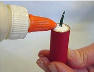
Insert the 1-1/2" piece of fuse (with the diagonal end sticking out) so about 1/2" is outside the shell.
