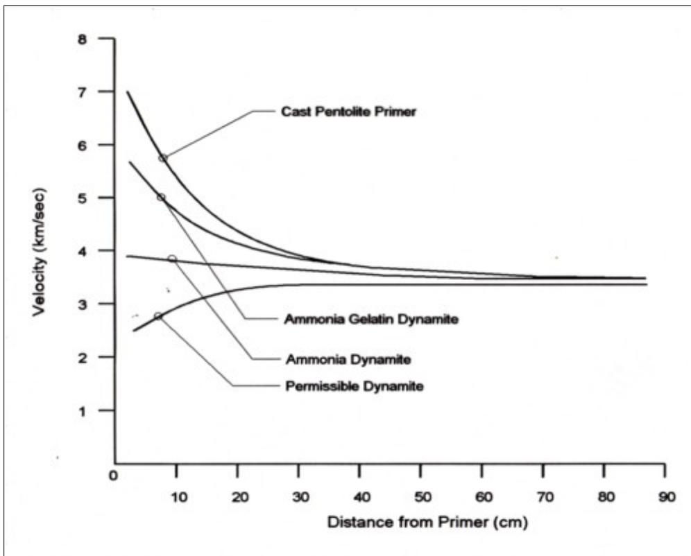
Detonation Velocity Transients Near Primer for a Variety of Explosive Products
