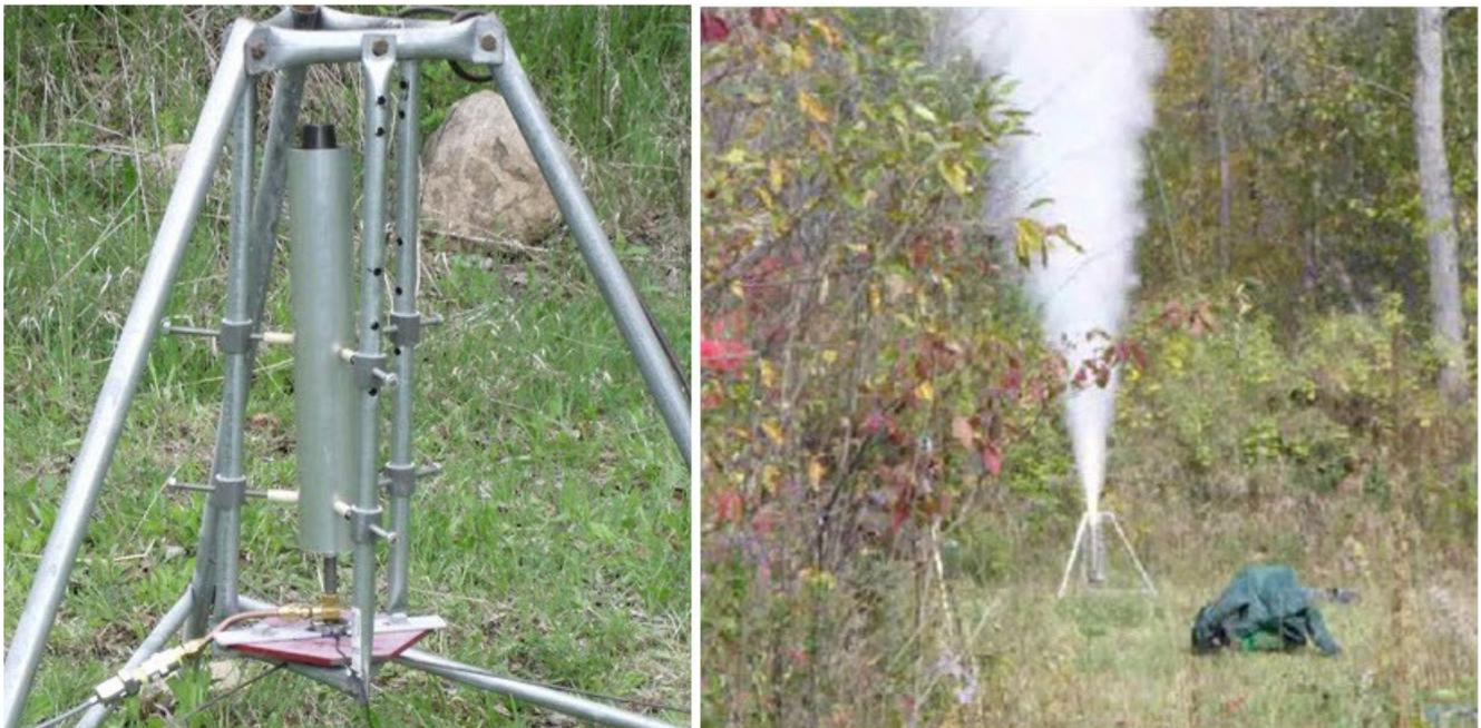
**Figure 13** -- A24-C1 rocket motor mounted in test stand (left); at full thrust (right)
