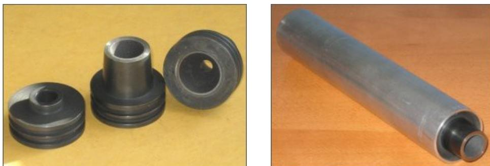
Figure 6 -- Nozzle assemblies and bulkhead for 38 mm motor, A24-B1 and A32-B1 static firings.
