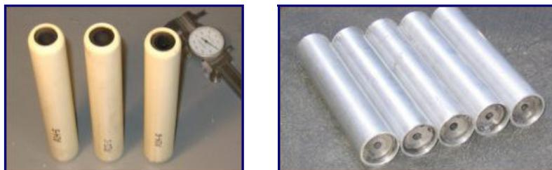
Figure 4 -- PVC motors (left) and aluminum motors (right) used for test firing AN formulations
