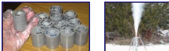
**Figure 10 -- A24 propellant grains for static tests; Firing of A24-B3 motor.**
