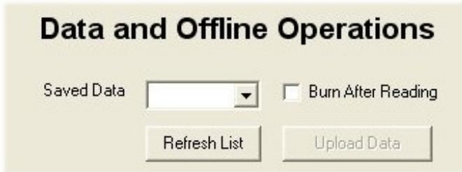
Clicking **Refresh List** sends a request to the rig to return a list of its memory contents. This will be returned as a list of run numbers, which are used to populate the drop-down box. When you select one, the **Upload Data** button becomes active, and clicking it will upload the stored data to the PC. This is held in memory, and also
