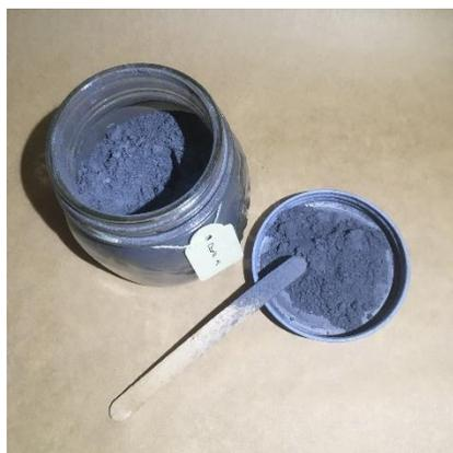
Spherical -200 Mesh Aluminium
